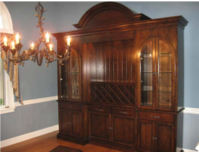
This arched-bonnet dining cabinet was built to designer specs, including a wine rack and arched doors - and interesting venture into circular work.
